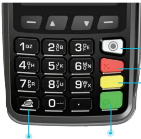
Feed paper a few centimeters if pressed for a long time (more than 2 seconds)
