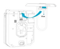
Use the adhesive tape of holder to fix it on the AXIUM RX7000.
