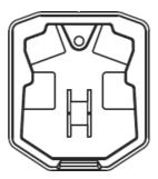
To fit the AXIUM RX7000 to the standpole, slide down the AXIUM RX7000 until a click sound:
