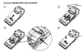
Note: Please put the cable to the correct position in the battery compartment, as the third picture shown
