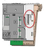
Slide back the module inside the terminal and screw it tight
